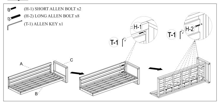
Place Back Rest (A), Seat Panle (B) and Right Frame (C) onto a padded, non marring surface. Attach Back Rest (A) to Right Frame (C) using with Short Allen Bolts (H-1) and provided Allen Key (T-1). Turn components as illustrated above. Attach Seat Panel (B) to Back Rest (A) and Right Frame (C) using Long Allen Bolts (H-2) and provided Allen Key (T-1). Do not yet fully tighten bolts.
