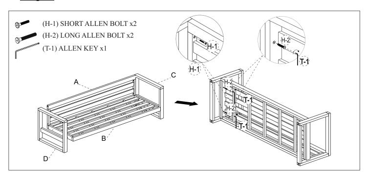
While Assembly from Step 1 is still on its back, attach Left Frame (D) to Back Rest (A) using Short Allen Bolts (H-1) and provided Allen Key (T-1). Then, attach Left Frame (D) to Seat Panel (B) using with Long Allen Bolts (H-2) and provided Allen Key (T-1). Fully tighten all Bolts from Step 1-2, but do not over tighten.
